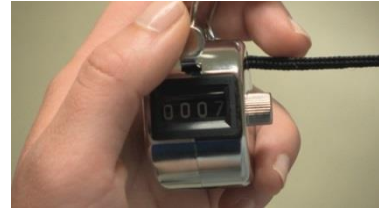
A mechanical lap counter can be used to count the number of lengths
